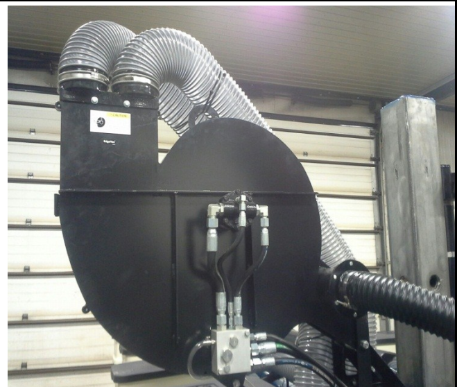
Figure 2. Fitting and tubes connected to the top of a Kinze planter (Kearney Planters, Highgate ON).
