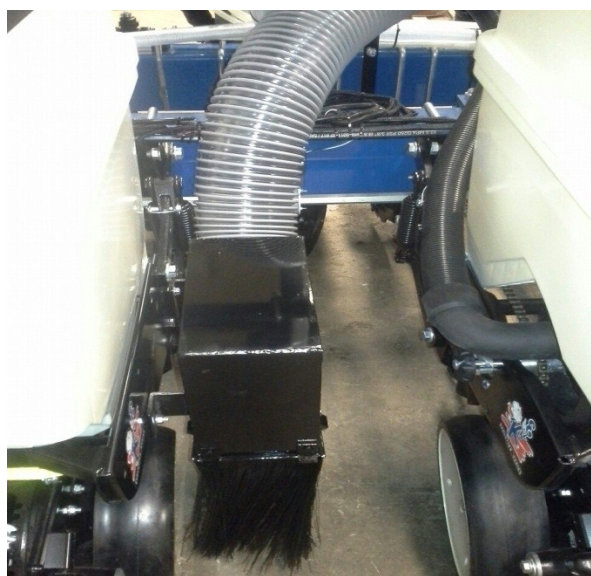
Figure 3. Expansion box and bristles to discharge air/dust (Kearney Planters, Highgate ON).
