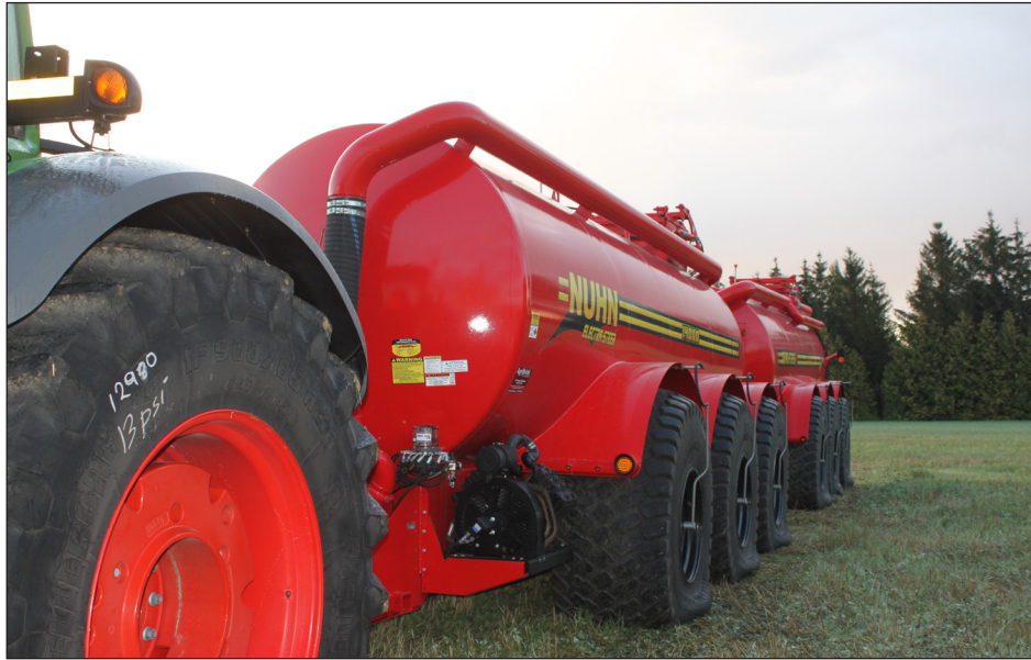
Figure 3. A manure tank with multiple axles, large tires and a centralized tire inflation system (CTIS).
