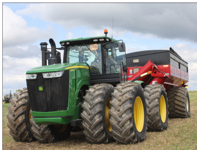
Figure 1. A tractor and grain cart. Reducing axle weight, increasing tire size and reducing tire pressure will lower the risk of compaction.
