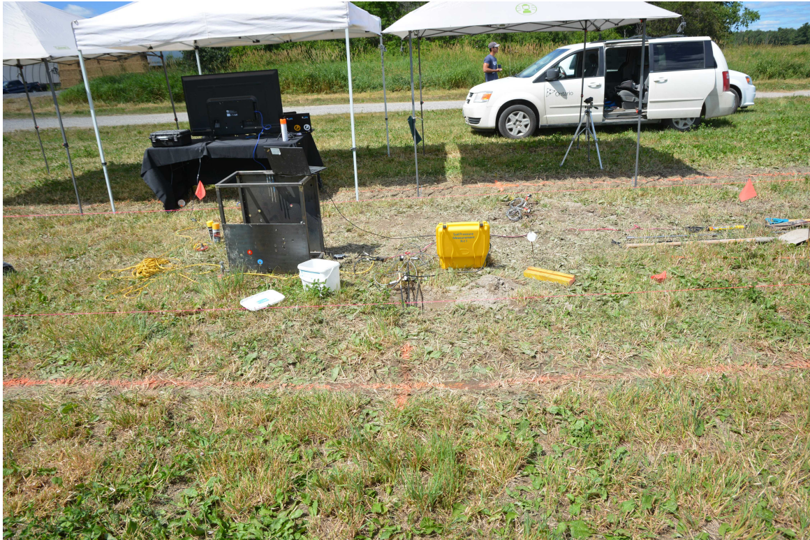
Figure 5: Installation of equipment for Bolling Probe pressure measurement
