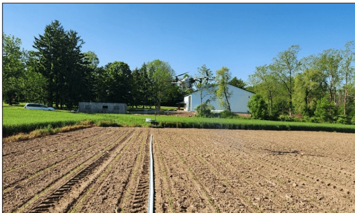
Figure 2. DJI T50 flying over sampling system to evaluate ESW on bare ground.
